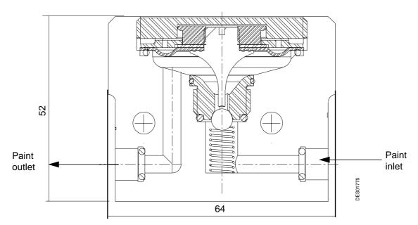
Note: The paint inlet and outlet are 1/8 iso threads.
